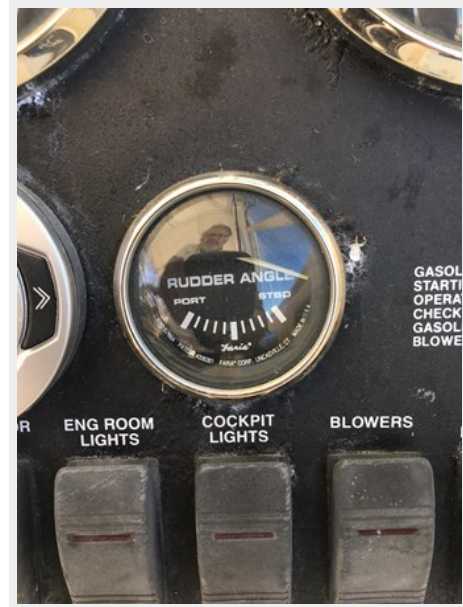
Rudder angle indicator
