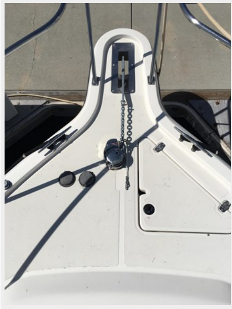
Windlass controls, anchor locker
