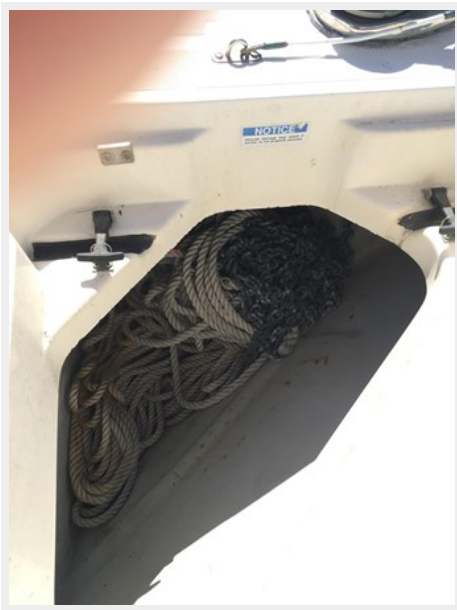
Anchor locker, chain/line rode
