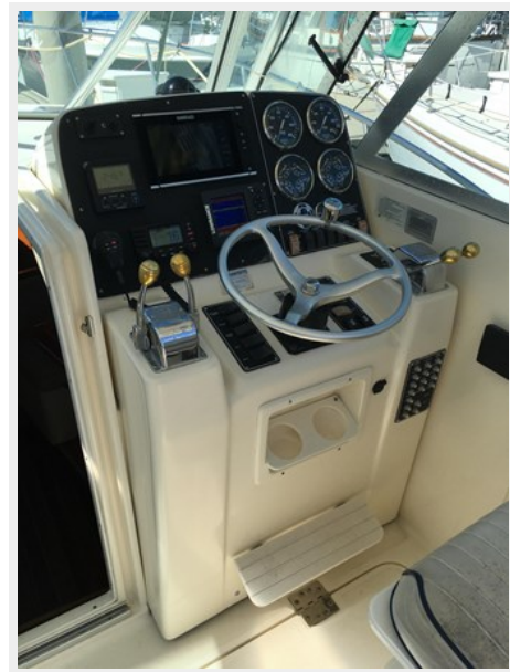
Modular helm, tilts aft for electronics access
