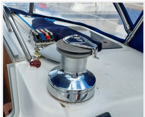
1021 All In Hunter 37.5 Cabintop Winch
