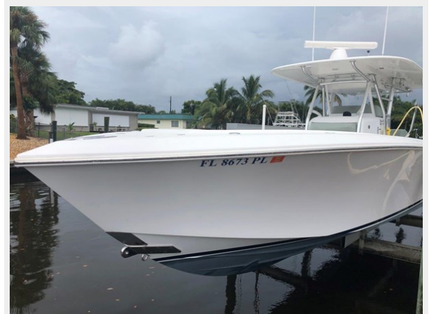
On the boatlift - Note towing eye
