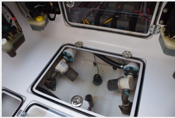
Sealed bilges hatches - livewell intakes
