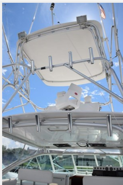
Tower FRP top with spreader lights
