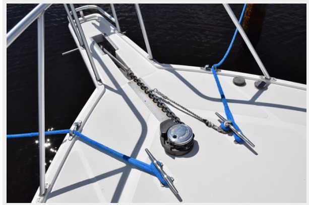
Electric windlass and pulpit with roller chute
