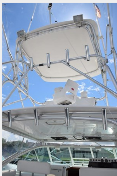
Tower FRP top with spreader lights
