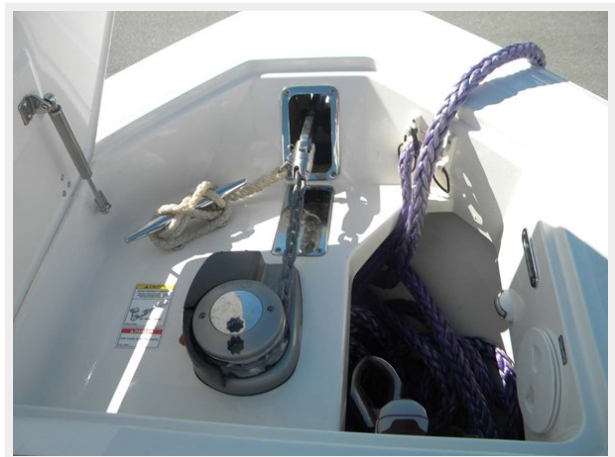
Anchor Locker, Windlass, Rode, Chain, Tow Line
