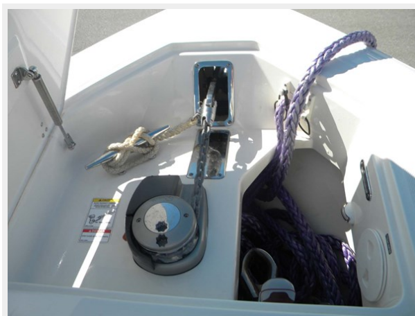
Anchor Locker, Windlass, Rode, Chain, Tow Line
