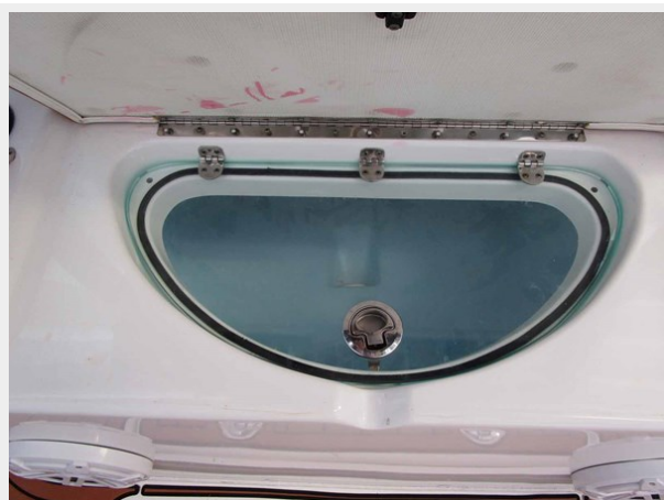
Live Well Under Aft Facing Seat
