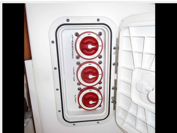
Engine Battery Switches
