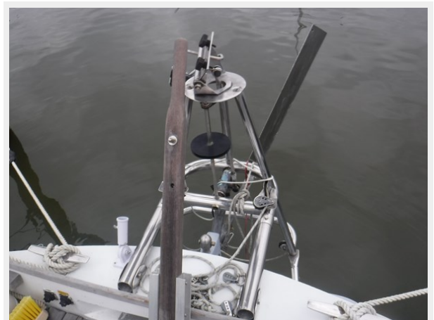
Wind Vane Self Steering system
