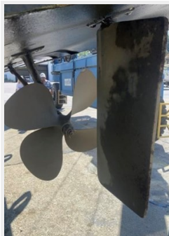
Starboard Rudder & Prop
