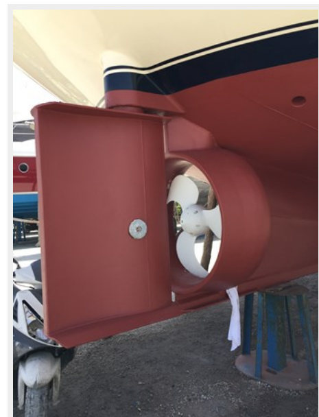
rudder, variable pitch prop and tunnel
