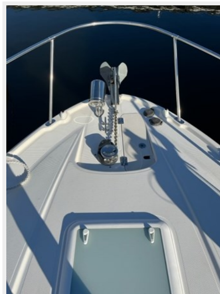
10 Windlass and Remote Spotlight
