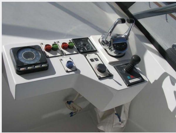
Flybridge Console to Starboard
