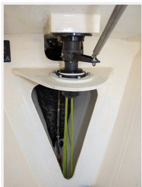
Under-deck Line Controls
