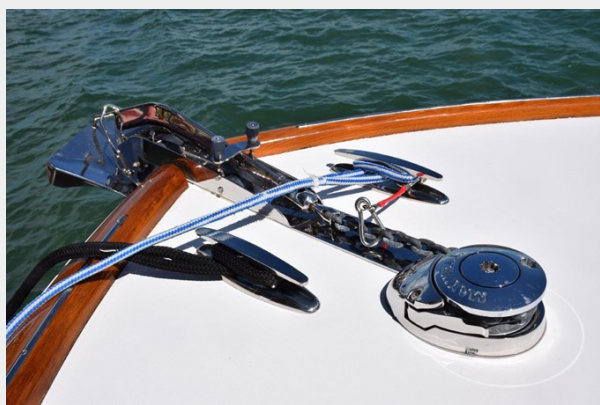
Electric windlass and stainless chute
