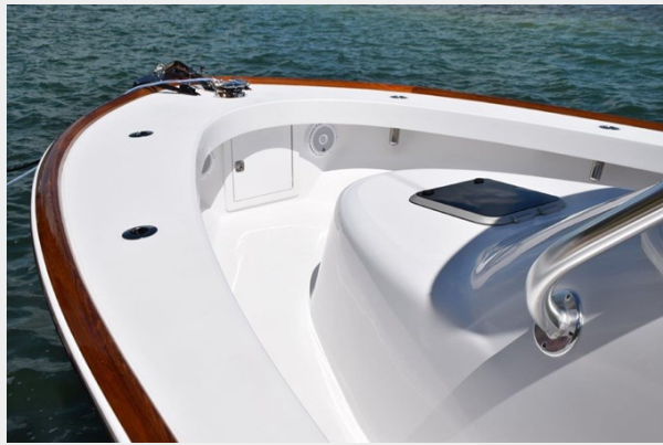
Varnished toe rail, full walk-around
