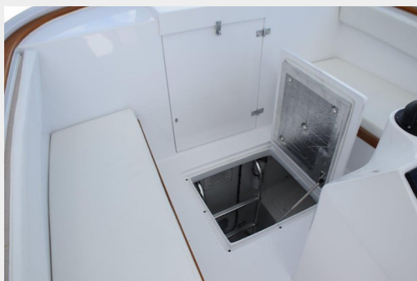
Engine-room drop down hatch
