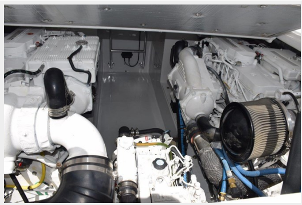
380hp Cummins QSB common-rail motors
