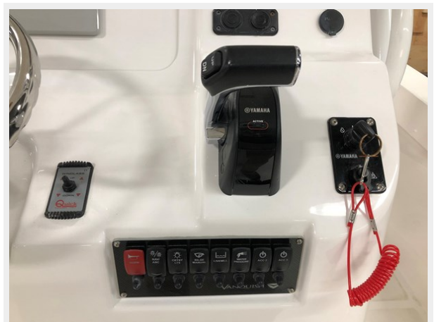
Throttle Controls and DC panel
