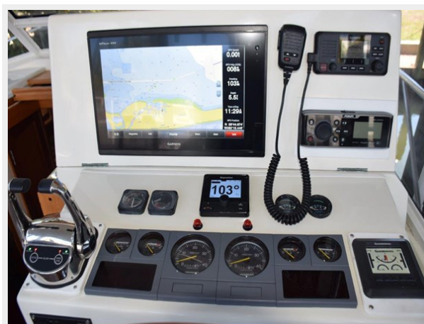
Helm with Garmin MFD, VHF radio, and autopilot
