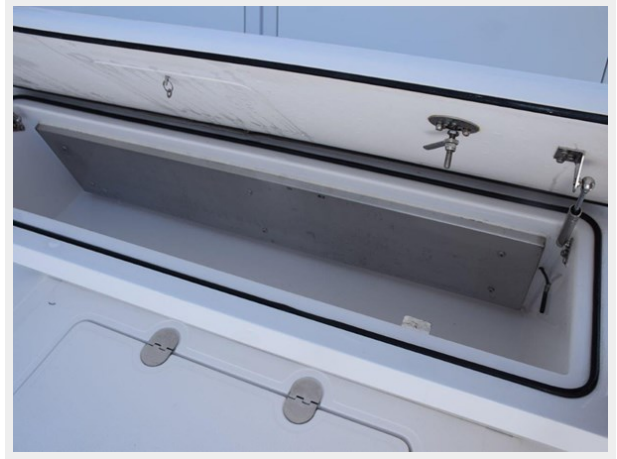
Refrigerated box beneath aft facing seat
