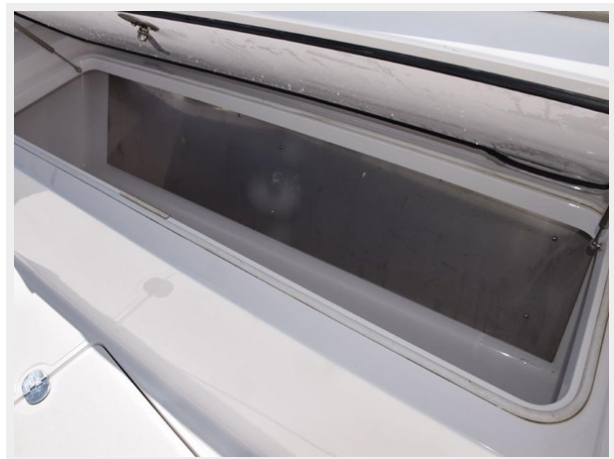
Refrigerated box beneath starboard forward seating lounge
