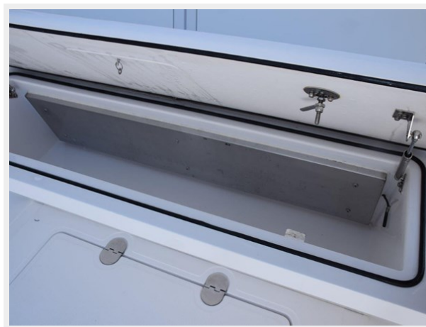
Refrigerated box beneath aft facing seat
