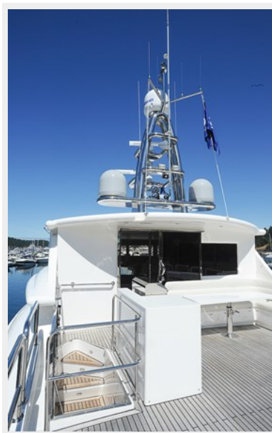
Custom Radar Arch
