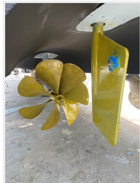
Port Running Gear
