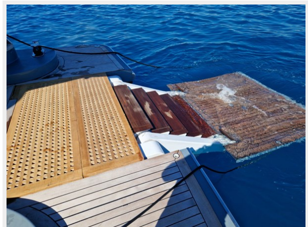
Swim platform transformer
