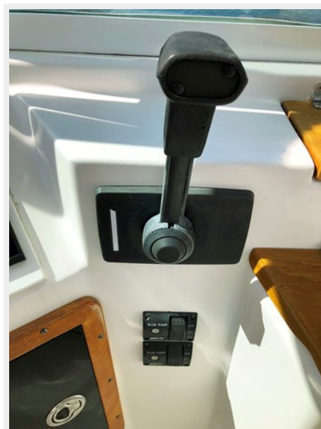
Sidemount Throttle and Shift
