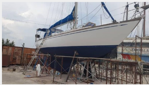
Refurb hull & underwater ship done
