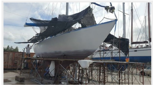
Refurb bow painted
