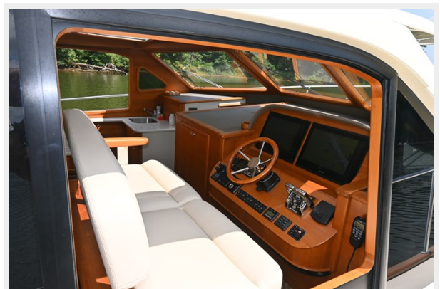
2020 Palm Beach 55 "Luce Lady" - helm from open side window. Allows captain to get on deck quickly
