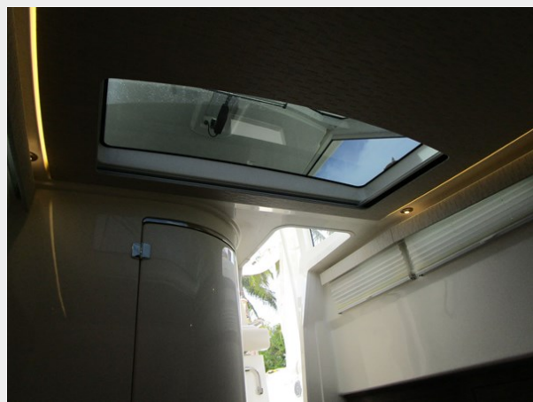
Overhead Dead Light
