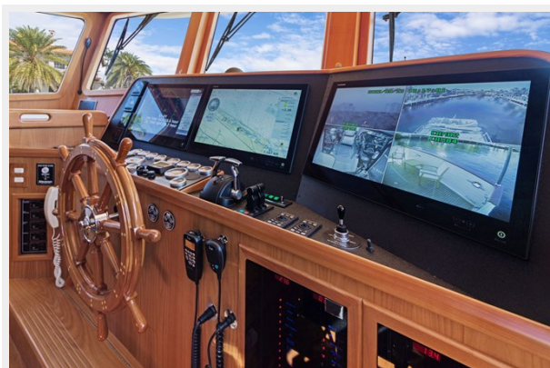
Pilothouse helm electronics
