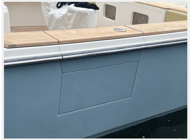
Dive Door Installed 8/2022
