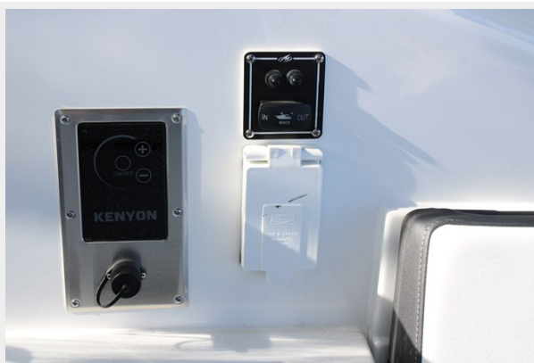
Cockpit Shade & Electric Grill Controls
