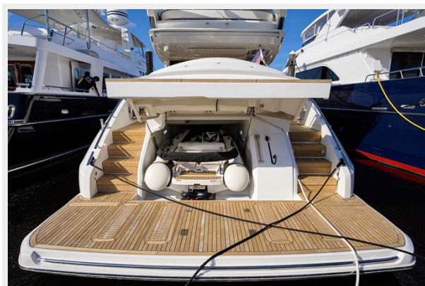
Swim Platform and Tender Storage
