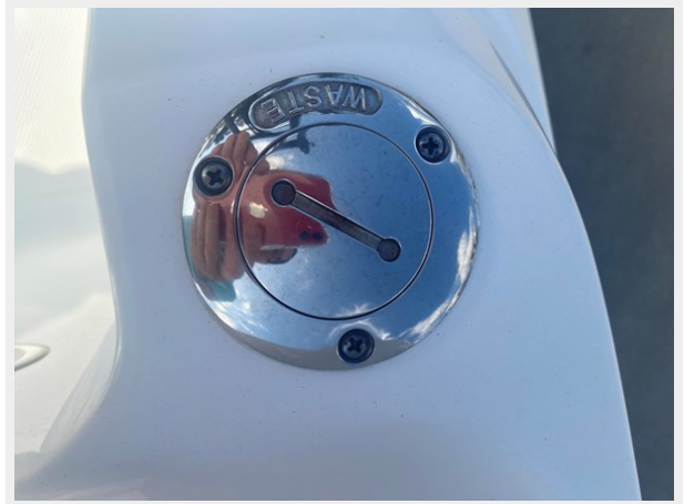
22-Waste Pump Out
