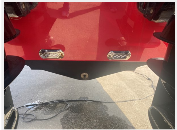
07-Under Water Lights
