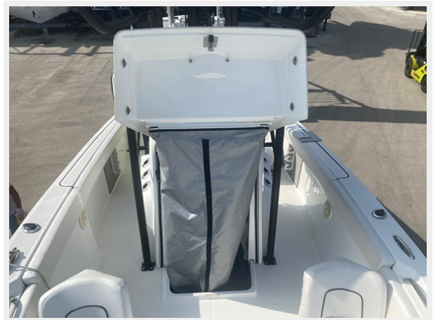
12-Head Compartment Enclosure
