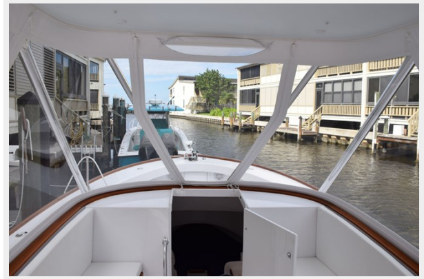
GG Canvas, Track to Track Fitted, Vent Panel Above Center
