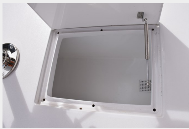
Macerated -Refrigerated Fishbox Behind Fighting Chair
