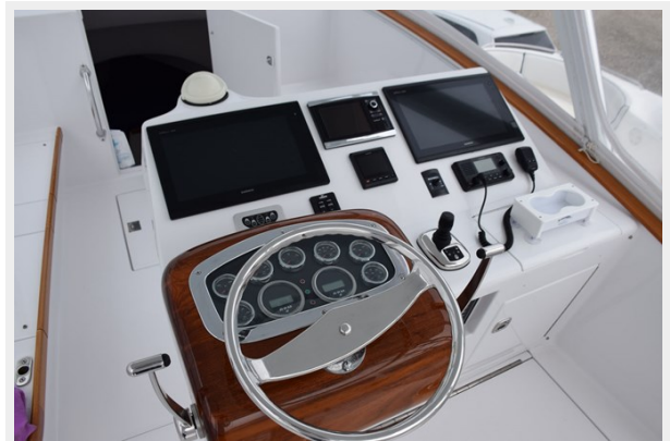
Teak Helm Pod, Thruster Control Button Single Levers, Joystick
