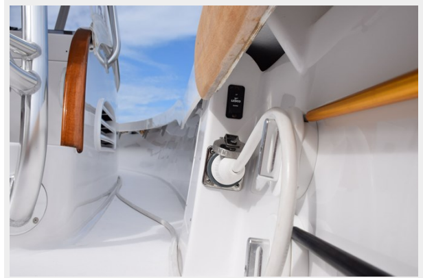
046 Walk-Around Side Decks, Engine Room Vents, Inboard Tower Legs 047 Secure Gaff Racks, Electric Lift Engine Hatch Switch
