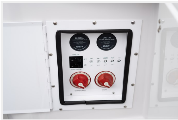
26. h290 battery switches
