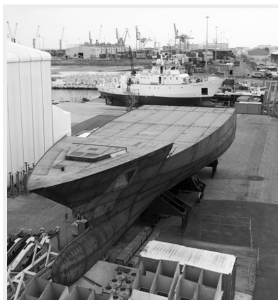
ISA CONTINENTAL 80 under construction
