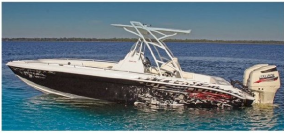
Built at the Glasstream yard in Panama City, Florida, the 280 ZS is a combination angling and pleasure center console that offers high-end performance with fishing amenities. The boat's stepped-bottom hull offers more deadrise at the transom and runs more than 70 mph when equipped with twin Suzuki DF300AP 300-horsepower engines. Power options range from the big Suzuki engines down to smaller 150-hp outboards, which still offer good performance and provide the safety of twin engines. Measuring 27-feet, 8-inch long, the Glasstream 280 ZS on display at the 2014 Miami International Boat Show was rigged with Suzuki Precision Maneuvering that allows the driver to dock with ease through to joystick control.
