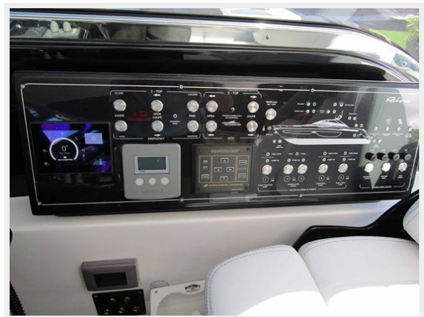
Helm Switches plus Seakeeper Controls
