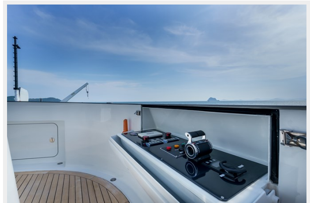
Wing control station on upperdeck
