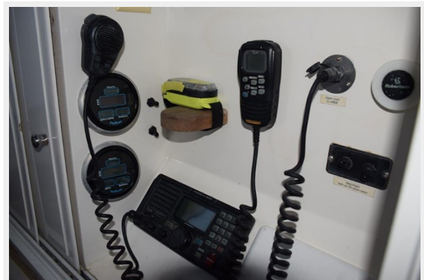
Flo-Scans and VHF Radios on Flybridge
