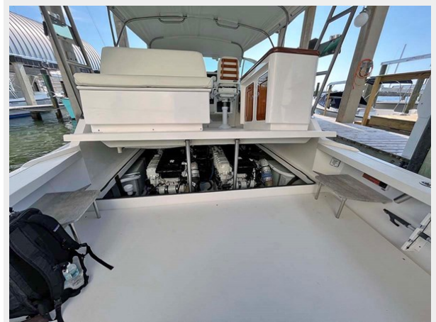
Lifting Bridge Deck
