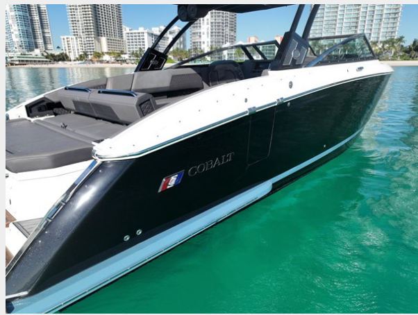
27 Stbd side boarding door
