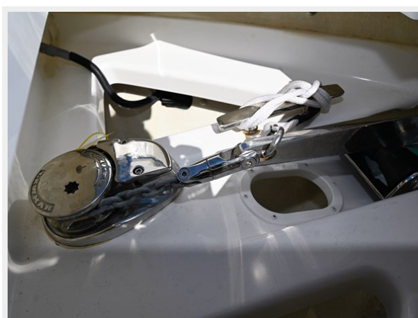
19 Bow electric Lewmar anchor system
