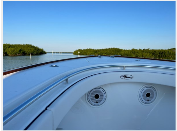
Toe rail combing bolster
