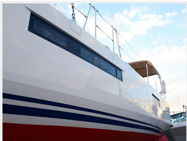
Topsides Detail w Hard Chine
