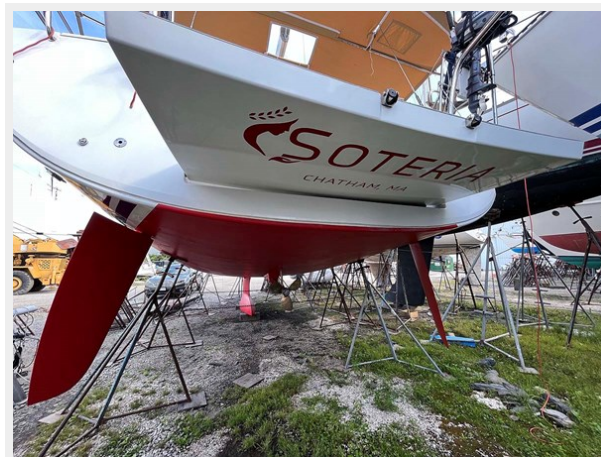
Fold Down Transom and Twin Rudders
