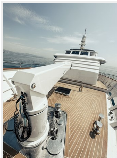
Bow Area - Tender Crane
