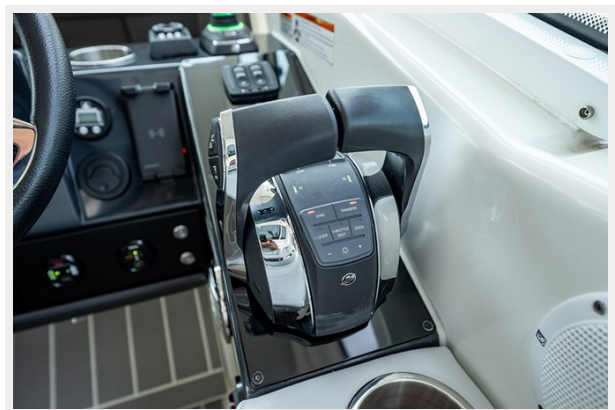
Mercury DTS control
