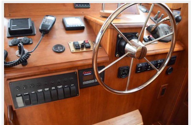
Lower helm switch panels
