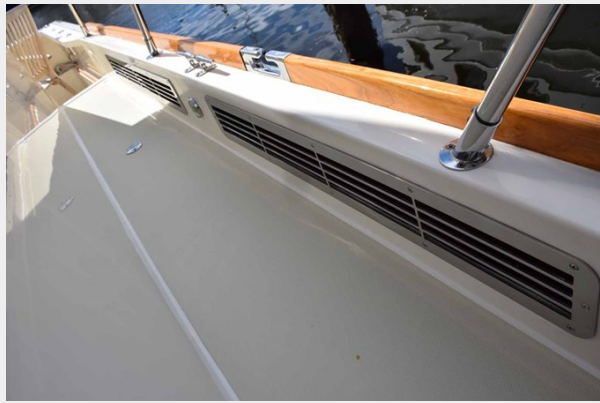
Toe railing and engine room vents
