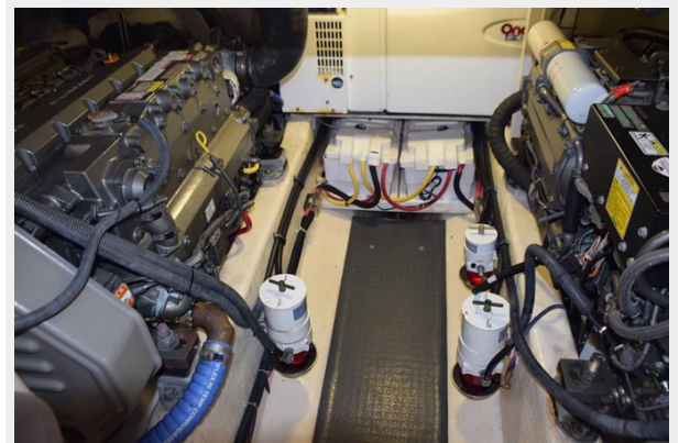
Yanmar diesels, 480hp each
