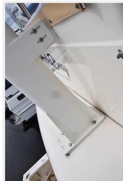
Hinged signal mast
