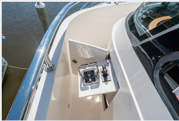
Fly Bridge Port Side Control Station
