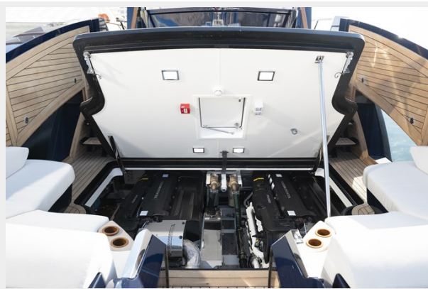
Engine room hatch
